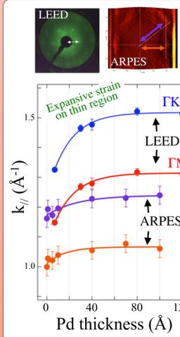
Fig. above: Those features are extracted value of  $k_{||}$ , depending on Pd overlayer thickness, in 2 dimensional electronic structure from LEED (upper one is for  $\Gamma$ K and lower one is for  $\Gamma$ M point, from geometrical position of spots), and ARPES (for 2 direction of symmetry lines as indicated arrows, from band dispersion and 2D mapping).
