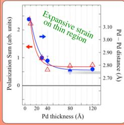
Fig. at left: The blue curve is the extracted values for Pd-Pd distance figured out from LEED images, and the red curve is the summed value of spin polarization of the range between  $E_F$  to 1eV, as graded on SPIPES results, referring to Pd thickness. The horizontal gray strap around thick Pd thickness is refereeing to the bulk Pd-Pd distance.
