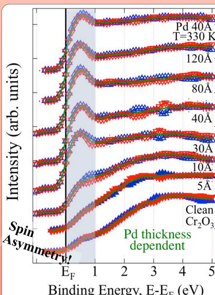
Fig. above: Experimental SPIPES results for clean  $\text{Cr}_2\text{O}_3$ , at bottom, and variety of Pd thickness on top of  $\text{Cr}_2\text{O}_3$ , at room temp. The very top feature is for  $T \approx 330$  K with 40 Å, for comparison.
