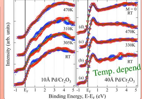
Fig. above: The results of temperature dependent SPIPES measurement of Pd thickness of 10 Å (left) and 40 Å (right) on  $\text{Cr}_2\text{O}_3$  (0001). The feature on right panel on the top, is for the result for zero external magnetic field applied on the 40 Å Pd on  $\text{Cr}_2\text{O}_3$  (0001) single crystal, at room temperature, for comparison.
